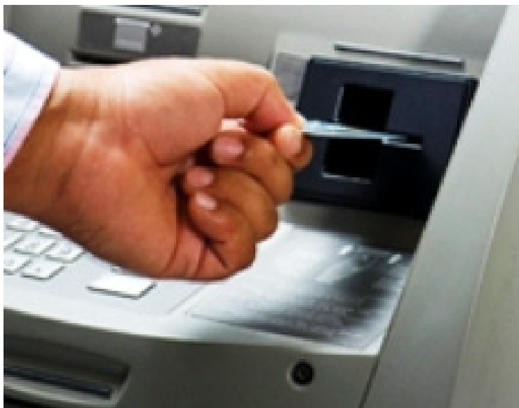
For independent ATM deployers, a major step in making the switch to EMV will be installing new hardware, including an EMV-enabled card reader.
