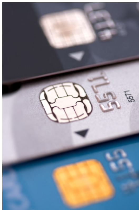
EMV cards contain a computer chip that is capable of securely storing data that uniquely identifies the card and authenticates the cardholder.
